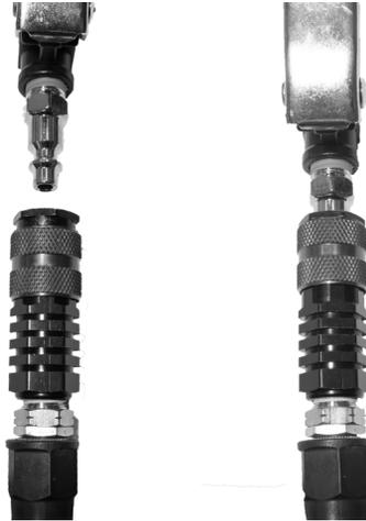
*Super Coupler* (black and silver) is auto-lock and you do not need to pull back the silver collar when coupling. When the silver collar is in the 'up' position, you can then slide the black collar to the 'up' position. The silver collar is used to lock the air tool in. The black collar acts as an 'on/off' switch for the pressure in your hose. Both must be fully in the 'up' position before starting to use your air tool.
